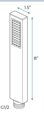
Flow Rate: 2.0 GPM / 7.6 LPM
